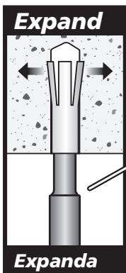
Expand anchor with the Red Head Setting Tool until shoulder of tool is flush with the end of the anchor.
