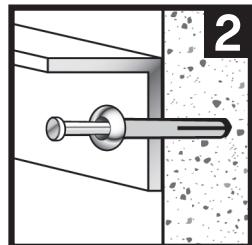
**Insert anchor until head of anchor body is flush with fixture.**
