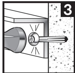
**Tap the nail flush with the head of the anchor.**
