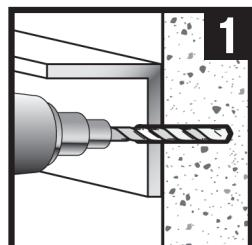
**Requires 1/4" Drill bit. Drill hole (through fixture) at least 1/4" deeper than anchor embedment.**
